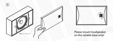
Mount the grill on the loudspeaker and set correct AMC logo direction.
