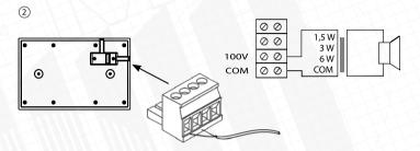
Connect audio cable to the Phoenix connector located on the rear panel. Power taps are marked near the connector.
